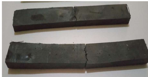
Figure 7. Results of testing specimens that have undergone flexural testing.
