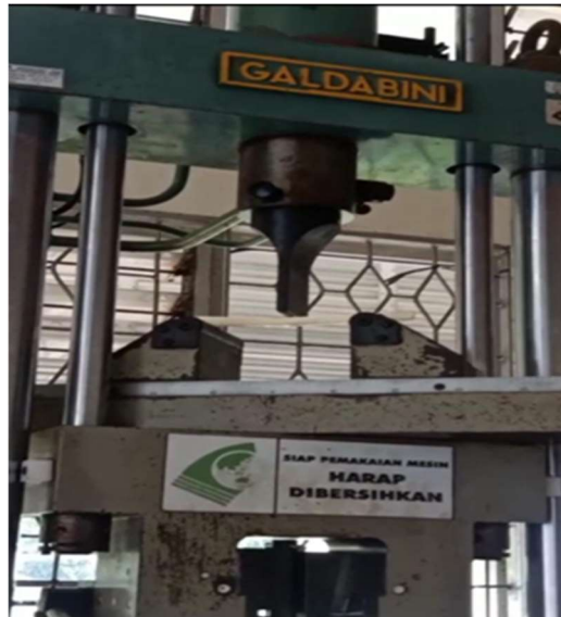
Figure 6. GALDABINI 32559 Series Flexure Testing Machine.
