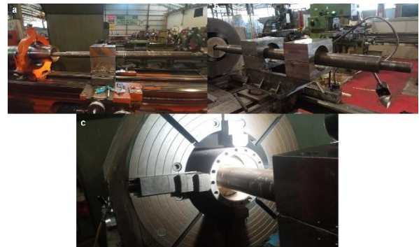
Figure 2. Variations of modification of double chuck which a. existing holder, b. new holder, and c. with wood
