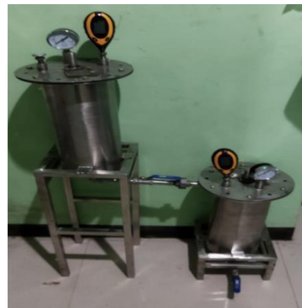
Figure 5. Two-stage anaerobic reactor apparatus
