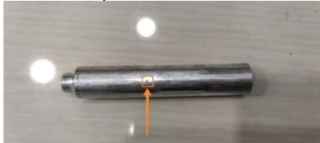
Figure 7. Leak in the tube
