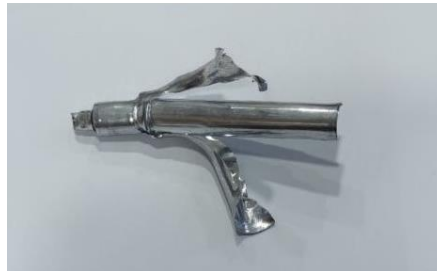
Figure 6. Extreme Damage to the tube
