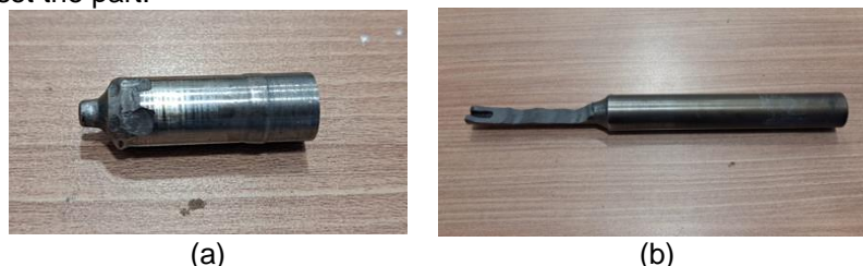
Figure 9. Figure (a) Stamp Damage, (b) Punch Damage
