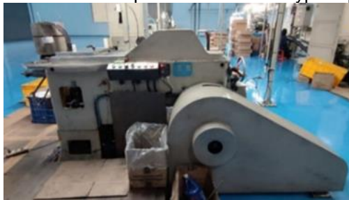
Figure 1. LJ-60 impact extrusion press machine (3D)
