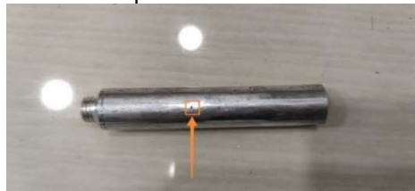
Figure 7. Leak in the tube
