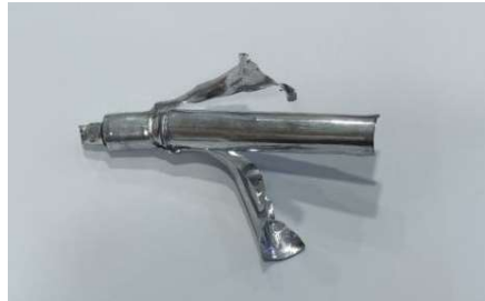
Figure 6. Extreme Damage to the tube
