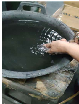
Figure 5. Tube Leak Testing
