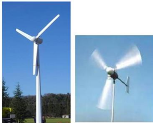
Figure 2. Horizontal-axis wind turbine
