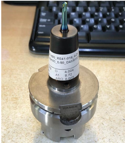
Figure 5. Cutting Tool Installed on Shrink Fit Tool Holder
