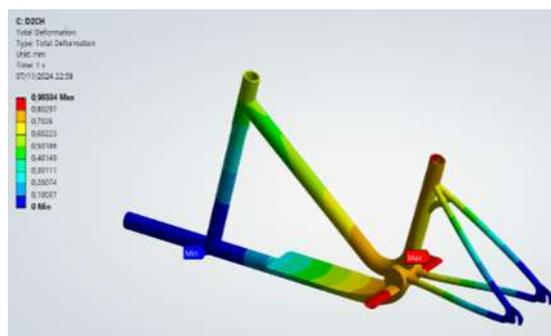
Figure 11. Deformation Design 2
