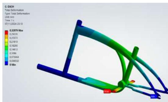
Figure 14. Deformation Design 3
