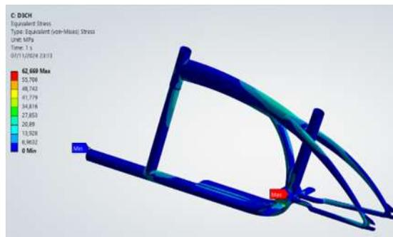
Figure 13. Von Mises Stress Design 3
