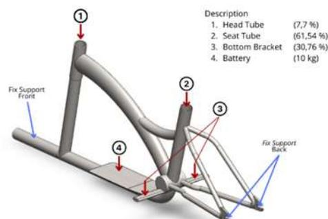
Figure 6. Loading Point and Fix Support
