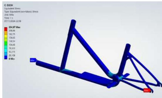
Figure 10. Von Mises Stress Design 2
