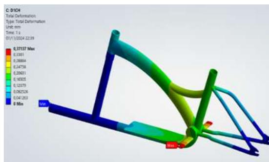
Figure 8. Deformation Design 1
