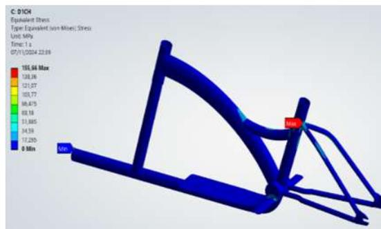
Figure 7. Von Mises Stress Design 1
