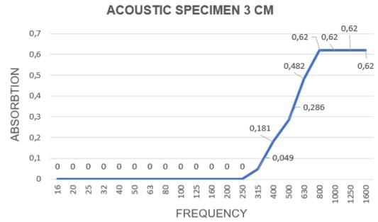
Figure 6. Acoustic testing of 3 cm specimen
