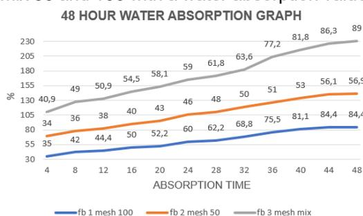
Figure 1. Water absorption 48 hours
