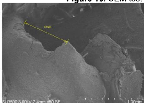
Figure 11. SEM test results of 50 mesh specimens
