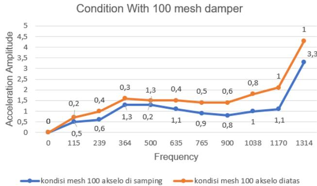
Figure 7. Vibration condition of mesh damper 100
