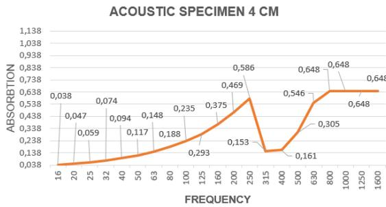
Figure 5. Acoustic testing of 4 cm specimen
