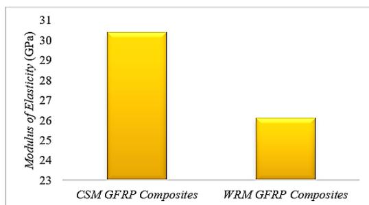
Figure 6. Comparison diagram of composite flexural modulus.
