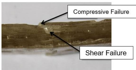
**Figure 8.** Flexural failure model of WRM GFRP (woven fiber composite)
