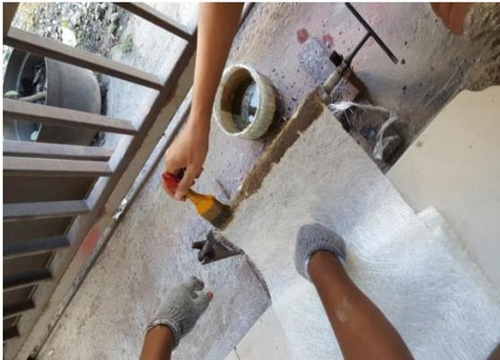
**Figure 1.** The process of applying resin to the fibers
