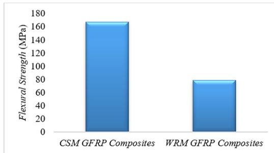
Figure 4. Comparison diagram of composite flexural strength
