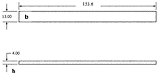
Figure 3. Flexural test specimen dimensions
