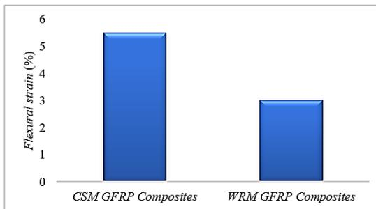
Figure 5. Comparison diagram of composite flexural strain.
