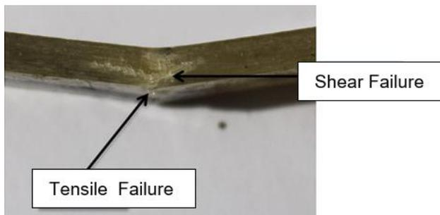
**Figure 7.** Flexural failure model of CSM/GFRP (random fiber composite)
