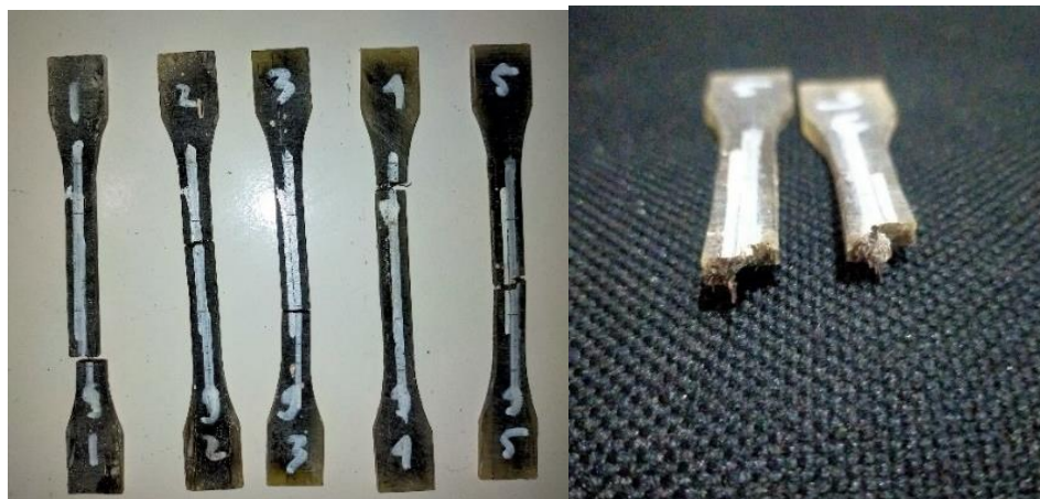
Fig. 3: Specimen failure content 9%
