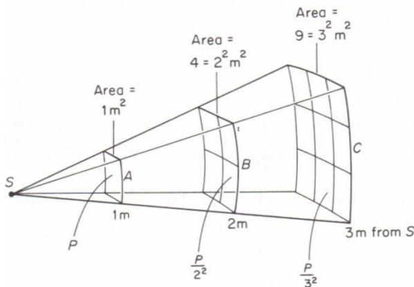
Fig. 26.20. Inverse square law for electromagnetic waves
