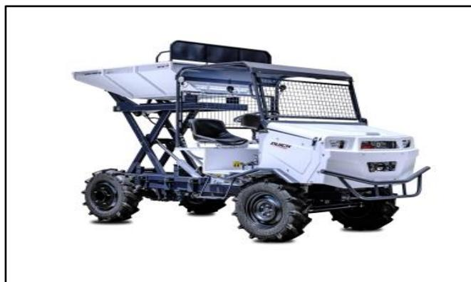
Gambar 4. *Tractor scissor lift*
