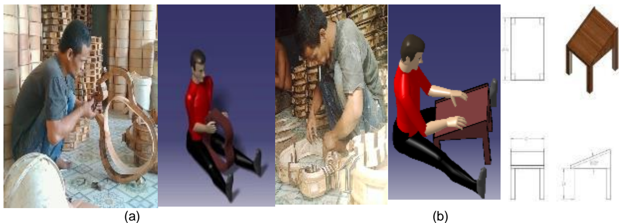
Fig. 2 Worker 3 (a) Body Side installation (b) Linnings installation.
