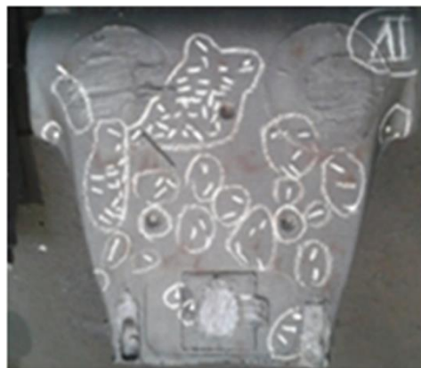
Figure 3. Defect sand inclusion on bracket products
