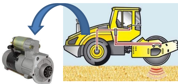
Fig. 1 Motor starter in compactor.
