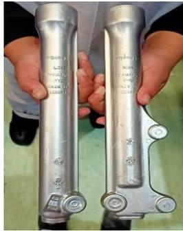
Gambar 1. Outer Tube Model 54P non gassing
