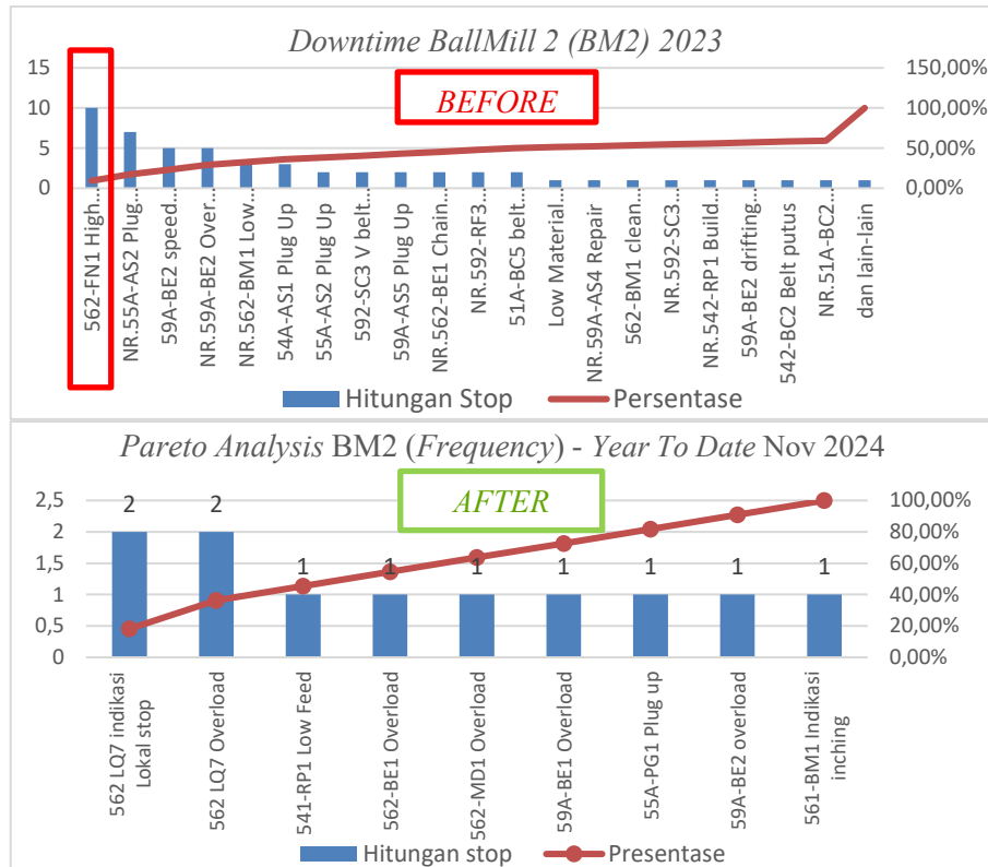
Gambar 8. Data Pareto After Pemasangan Automatic Cleaning Blade
