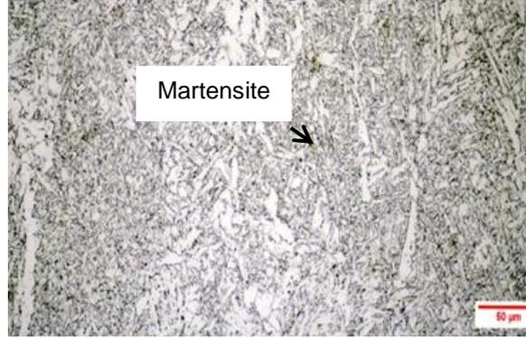
Figure 7. Microstructure at weld metal without WPS
