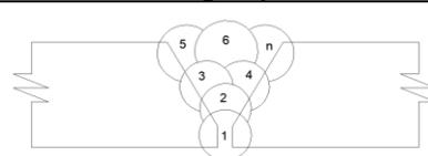
The WPS was made based on AWS D1.1 2015 standard, and the welding parameter could see in Table 3 and Table 4, respectively [21, 22, 23, 24]. Based on the WPS of line pipe material 8" API5L Gr X52, each base metal is defined in the AWS group number.
