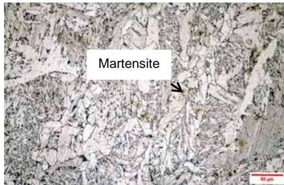
Figure 8. Microstructure at weld metal with WPS
