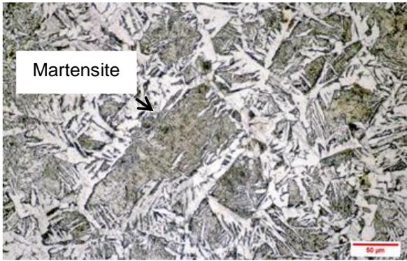
Figure 6. Microstructure at HAZ with WPS
