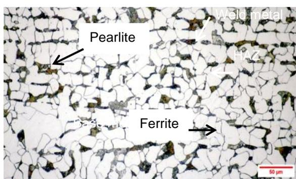
Figure 4. Microstructure photos of base metal
