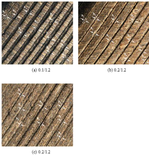
Figure 14. After contact, the gasket's surface roughness is 0-MPa for Ra 2.5 m.
