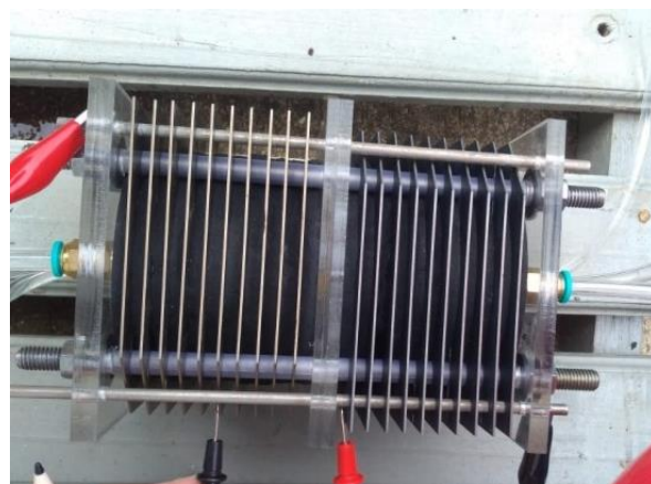
Figure 3. Photograph of HHO Generator
