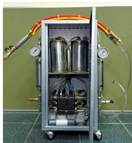
Figure 6. Prototype of HHO-based welding system
