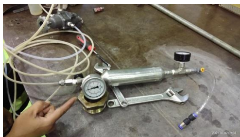
Figure 4. Pneumatic test setup for HHO gas storage cylinder
