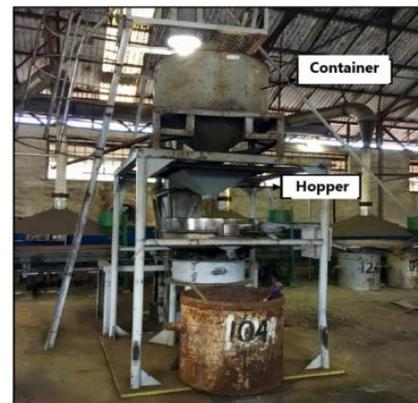
Figure 3. Round Screen for sieving air table middling to obtain – 20 mesh.
