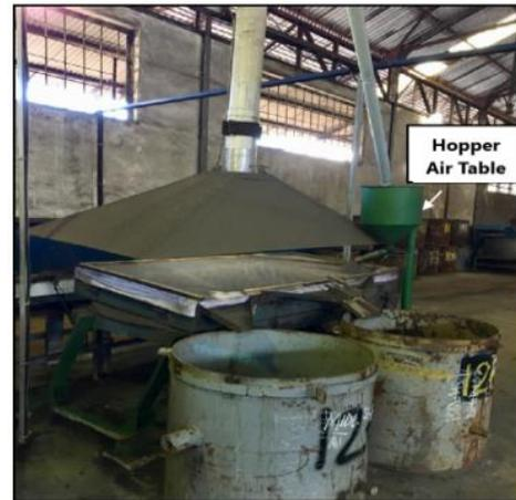
Figure 2. Air table for mineral dressing in Bangka Tin plant.
