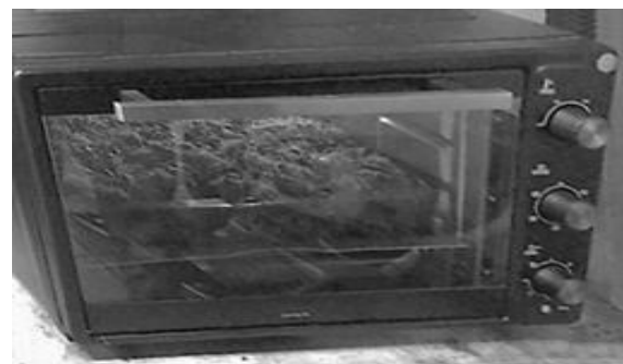
Figure 2. EFB Drying Process with an Oven
