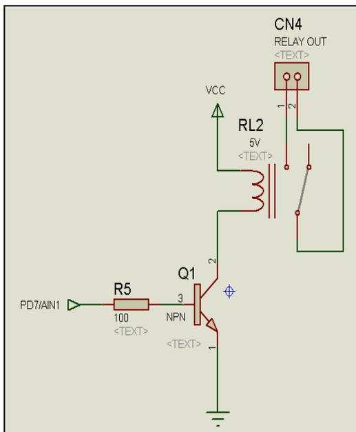
Gambar 7. Rangkaian ON/OFF power switch
