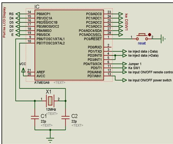
Gambar 6. Rangkaian Sistem Minimum Mikrokontroler ATmega8
