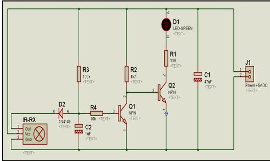
Gambar 9. Rangkaian IR Receiver Pada ON/OFF Remote Control
