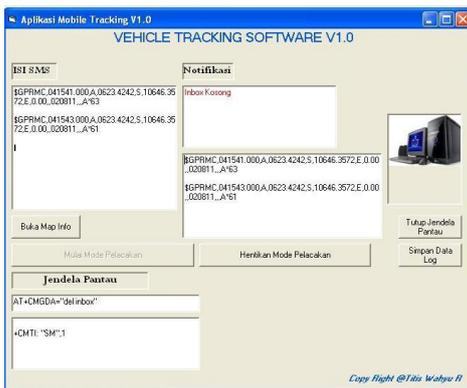
**Gambar 4.1 Contoh GUI Pengujian Mode Tracking. Saat Menerima data GPRMC**
