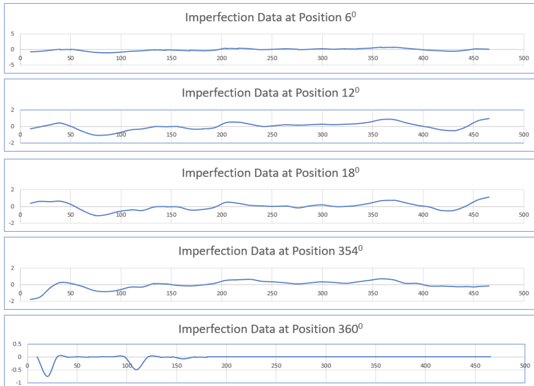
Figure 7. Longitudinal imperfection of some section (6°, 12°, 18°, 354° and 360°)
