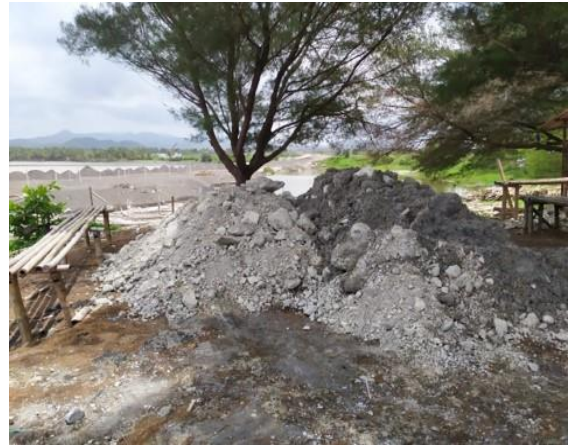
Figure 1. The deposited dried mortar waste at the batching plant location
