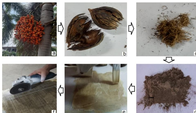
Figure 1. Flow chart of the composite fabrication process: (a) Foxtail palm tree with ripened fruits; (b) Dry tree fruits; (c) Fiber extracted; (d) Fibers converted to micro level (powder); (e) Reinforced in polymer; and (f) Cutting of specimen as per ASTM standards
