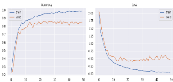
Figure 12. Accuracy-Loss Graph of the MobileNet model.
