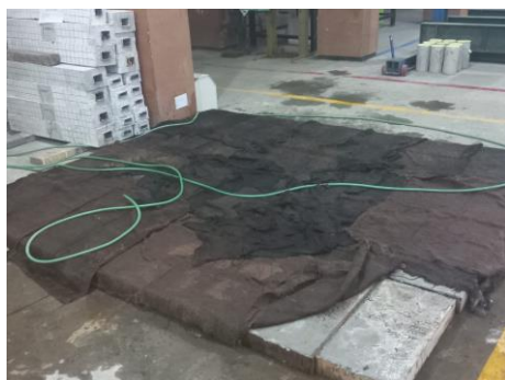
Figure 3. Ferrocement Specimen with Dimension 60x30x5cm
