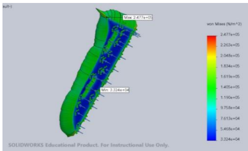
Figure 11. Finite element analysis of part 6, lateral support of the AFO design
