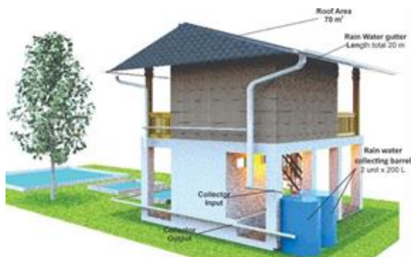
Figure 2. A design of harvested rainwater (RWH-1) with collecting drums at a wooden house. The water also channeled to CW-1, CW-2 and a fishpond
