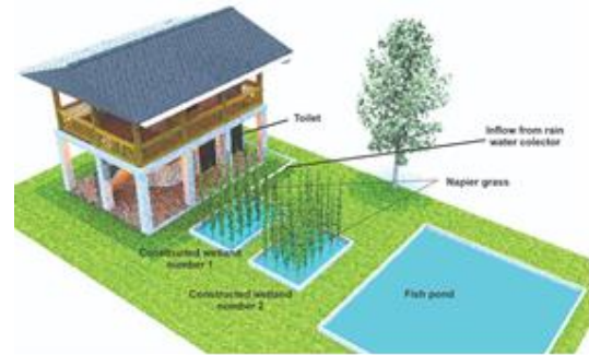
Figure 3. Technical design of a tiered constructed wetlands (CWs) with a fishpond. The source of the water is from rainwater and grey water
