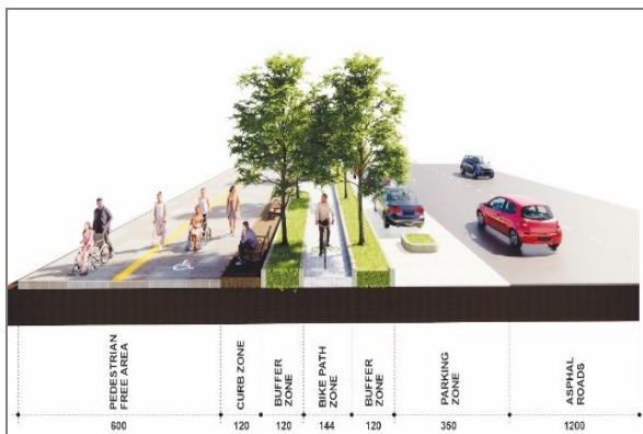
Figure 6. View of Model 1 Pedestrian Lane for Arterial Road
