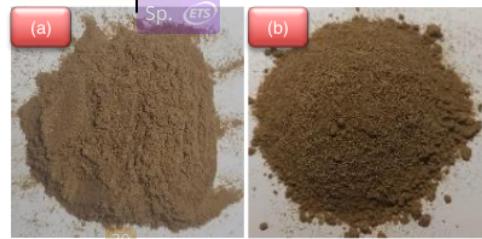
Figure 1. Water Hyacinth Powder: (a) Before, (b) After Activation
