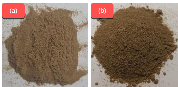
Figure 2. Water Hyacinth Powder: (a) before, (b) after Activated
