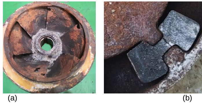
Figure 13. Impeller (a) and H-type Rubber Clutch (b) Conditions
