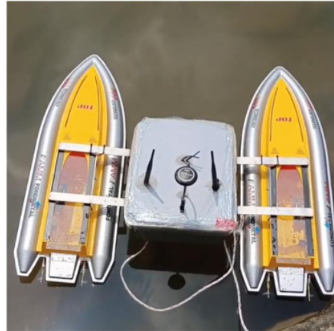
Figure 5. Hardware Design of Unmanned Surface Robot
