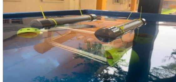
Figure 12. ROV Prototype Achieve Above 94% Negative Buoyancy
