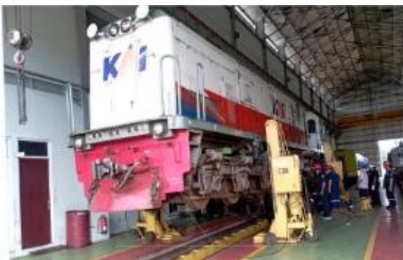
Figure 2. Lifting jacks for locomotive maintenance
