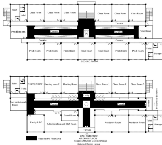
Figure 5. Selected design layout illustrating the integration of responsive human-centered design strategies and the placement of potential piezoelectric floor areas
