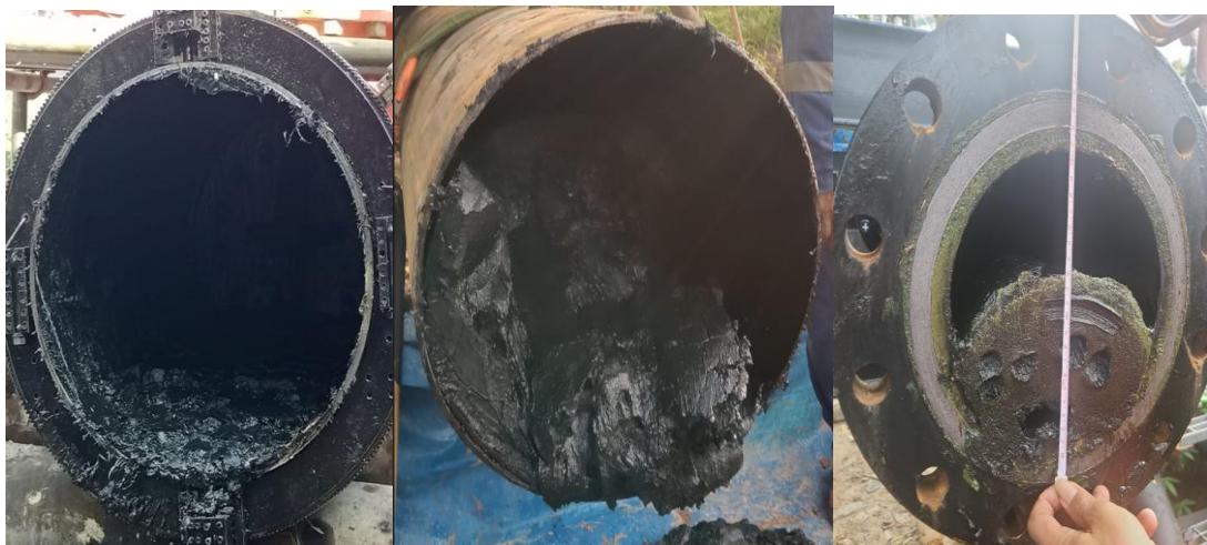
Figure 1. Wax deposit in a 24-inch pipe
