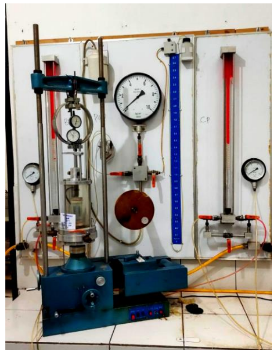
Figure 4. Consolidated Undrained (CU) triaxial compression test apparatus
