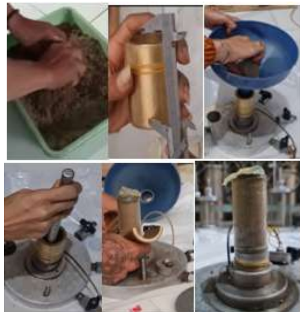
Figure 3. Specimen preparation using the moist tamping (undercompaction) method
