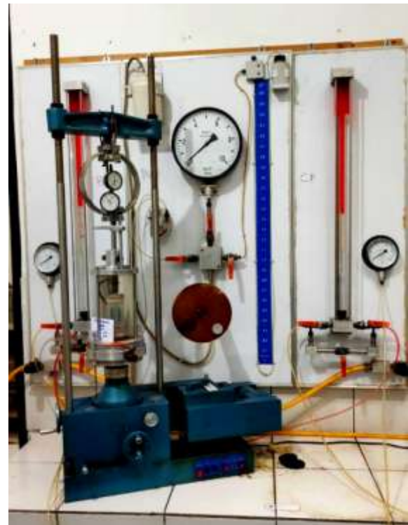
Figure 4. Consolidated Undrained (CU) triaxial compression test apparatus
