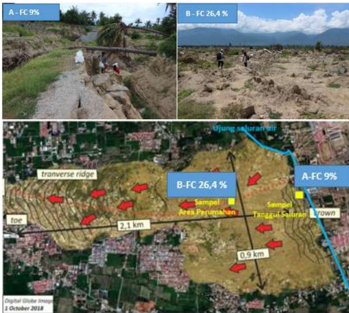
Figure 1. Sampling locations in Petobo: (a) drainage dike (Location A), (b) area affected by massive ground flow (Location B), (c) overview of the flow liquefaction-affected zone
