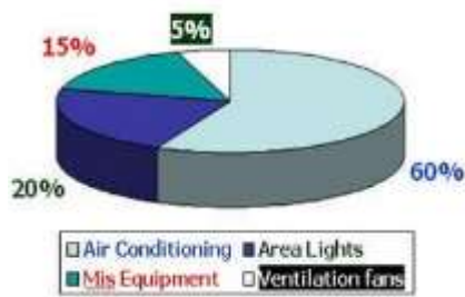
Figure 2. Typical Energy Consumption Pattern in Buildings: Typical Energy Saving Approach in Buildings (Hardik, 2015)
