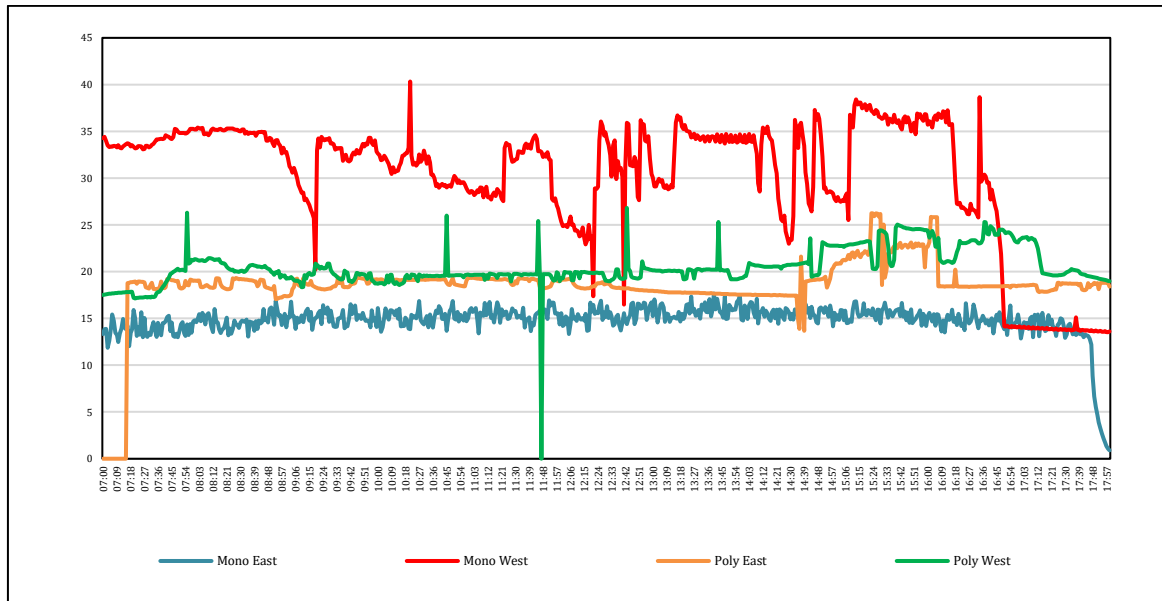
Figure 7. the 200-WP solar panel's temperatures and its output voltages in the East measurement
