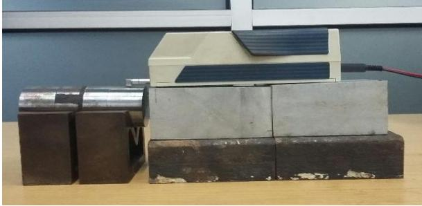
Figure 5. Surface Roughness Measurement
