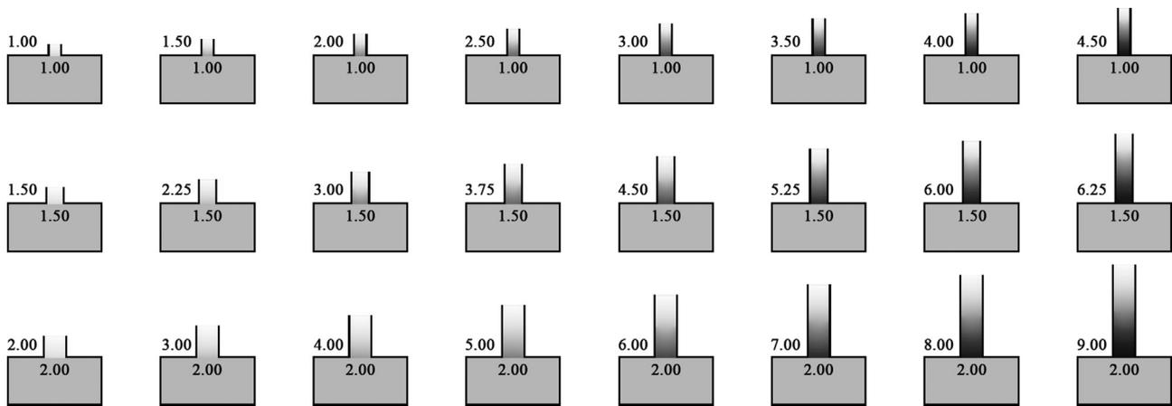
Fig. 2. Trial 1: variation in size and height/width ratio of the lightwell skylights.
