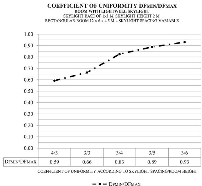
Fig. 7. Trial 4: coefficient of uniformity: quotient of the minimum daylight factor divided by the maximum on the work plane, with room length ranging between 4 and 9 m.
