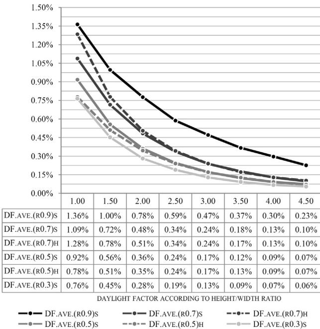
**Fig. 5.** Trial 2: average daylight factors (DF.ave.) on the work plane according to simulation software (S) and hypothesis (H). Variable reflection index and height of the skylight.
