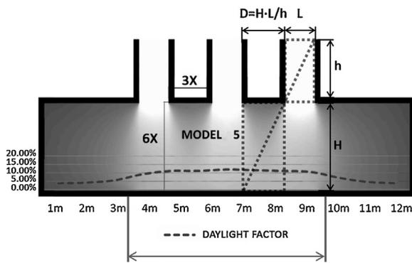
Fig. 8. Trial 4: skylight spacing according to width/height ratio of the lightwell.
