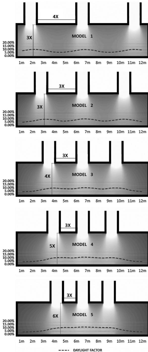
Fig. 6. Trial 4: daylight factors within a room in overcast sky conditions with lightwell skylights with a height/width ratio of 2/1. Variable spacing of the lightwells.
