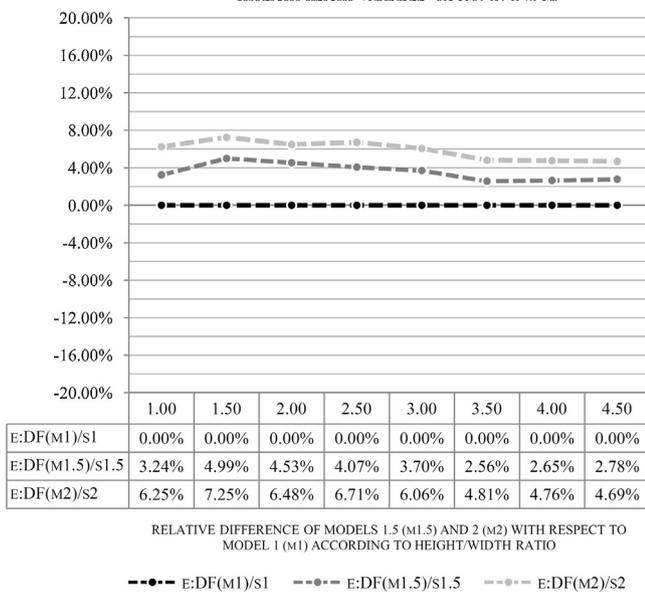
**Fig. 4.** Trial 1: relative difference of the quotient of average daylight factors on the work plane and the surface base of the skylight, according to simulation software. Models 1.5 (M1.5) and 2 (M2) with respect to model 1 (M1). Variable size and ratio of the skylight.
