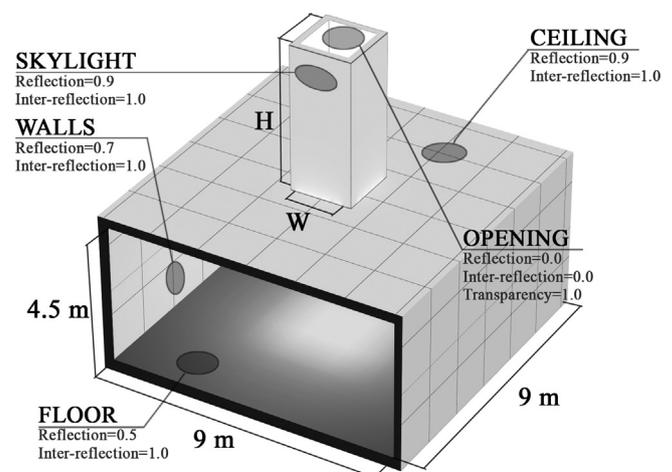
**Fig. 1.** Initial calculation model.
