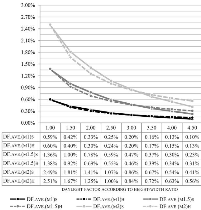
**Fig. 3.** Trial 1: average daylight factors (DF.ave.) on the work plane according to simulation software (S) and hypothesis (H). Variable size and ratio of the skylight.
